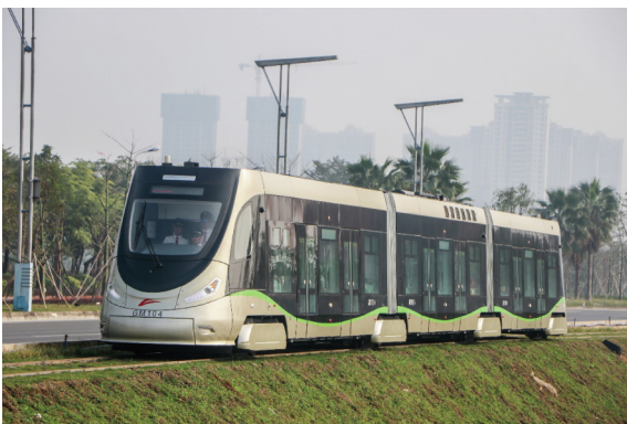
Fig. 2. Hydrogen-powered trams built jointly by Canada's Ballard Power Systems and China's CRRC Sifang are currently operating in the Chinese cities of Foshan (above) and Tangshan. Credit: Wikimedia Commons (CC BY-SA 4.0).
