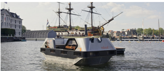
Fig. 1. A Roboat steers around an obstacle during a test run in Amsterdam in 2021. The 1200 kg craft, propelled by four electric motors, can carry up to five passengers or 1500 kg of cargo. Credit: Pietro Leoni/MIT (public domain).
