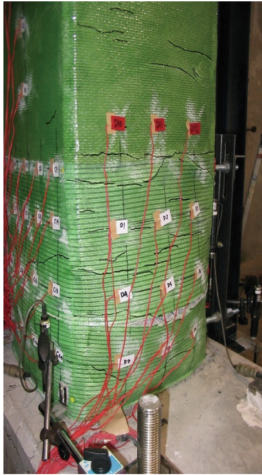
Fig. 2. A PET fiber sheet jacket showing high deformation without fracturing.
