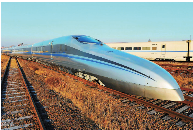
Fig. 3. New test model of 500 \text{ km}\cdot\text{h}^{-1} super high-speed train. Photo was provided by CRRC Corporation Limited.
