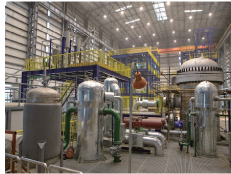
Fig. 3. The HTR-PM engineering laboratory at the Institute of Nuclear and New Energy Technology (INET) and a 10 MW th helium engineering test facility.
