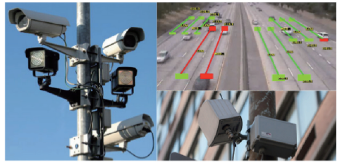
Fig. 2. Roadside units capturing real-time traffic situations and communicating with vehicles.
