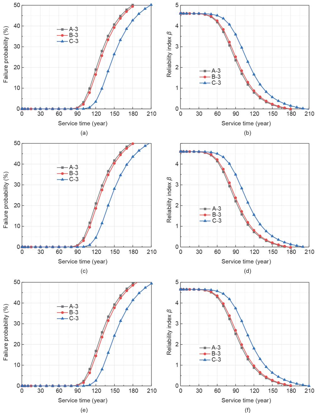
Fig. 13. Corrosion probability of steel and reliability index in different service environments: (a, b) splash zone; (c, d) tidal zone; and (e, f) underwater zone.
