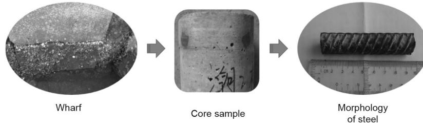
Fig. 7. Corrosion status of steel in a concrete wharf with a service age of 40 a in Dalian.
