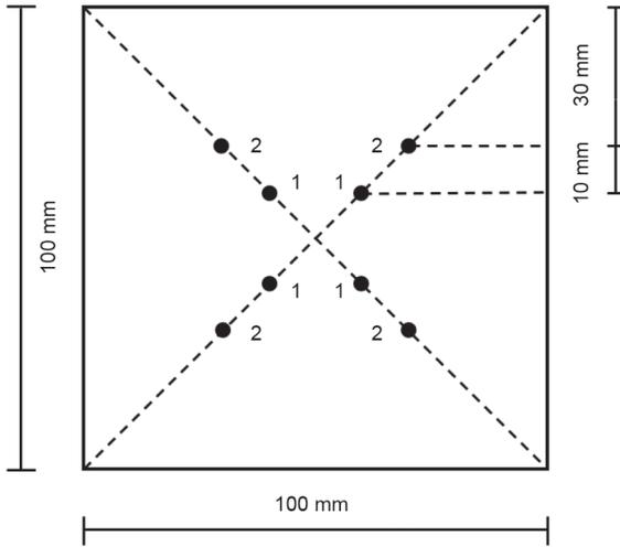
Fig. 3. Sampling locations of specimens.
