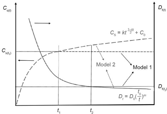
**Fig. 14.** Different time-varying relationships of boundary conditions and diffusion coefficient.
