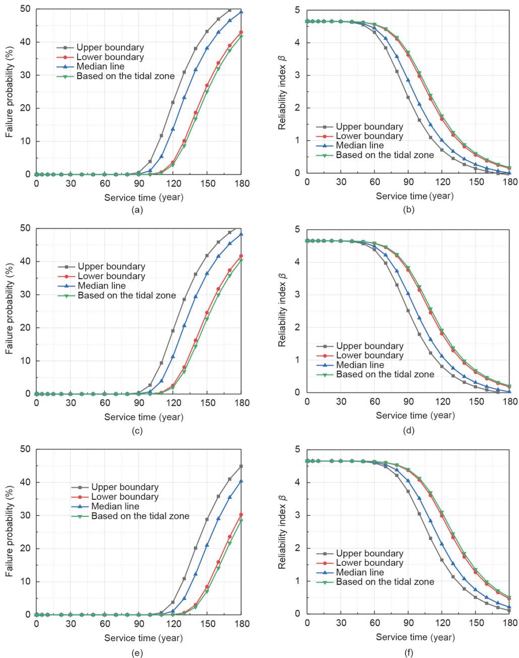
Fig. 18. Corrosion probability and reliability index of concrete structures under different boundary conditions: (a, b) A-3; (c, d) B-3; and (e, f) C-3.
