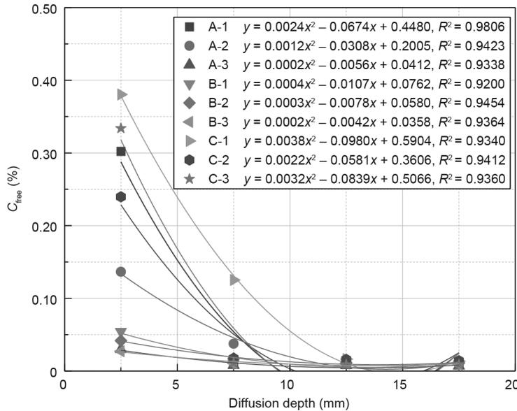
Fig. 4. Diffusion of  $C_{free}$  under indoor natural diffusion conditions.
