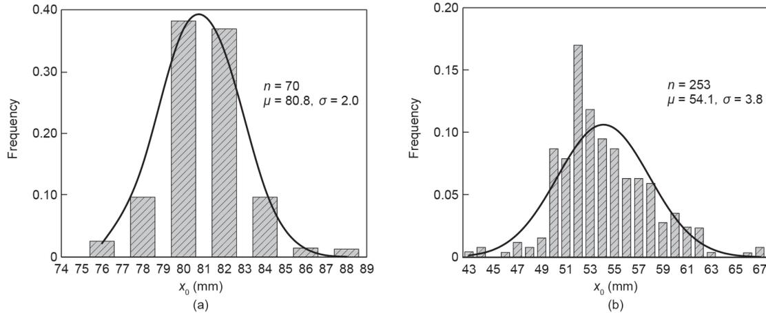
Fig. 10. Quality control level for different design cover thicknesses: (a) 80 mm and (b) 50 mm.  $\mu$ : average value;  $\sigma$ : standard deviation.
