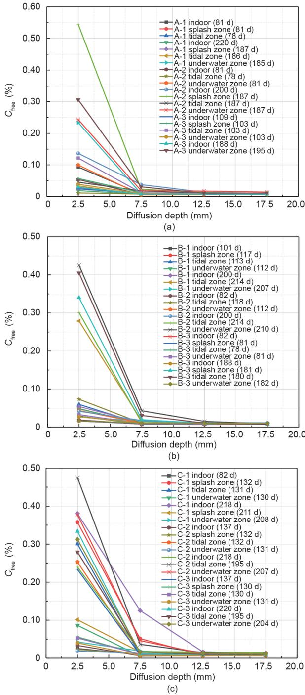
Fig. 8. Chloride diffusion in concrete under different exposure environments. (a) A series; (b) B series; (c) C series.
