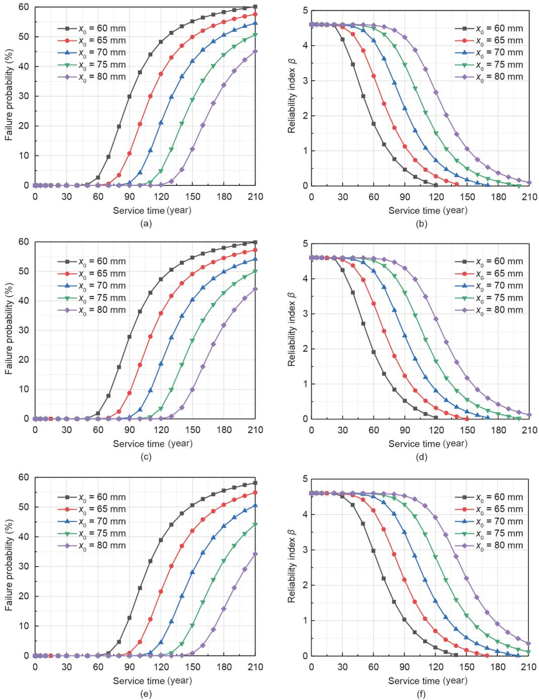
**Fig. 16.** Comparison of corrosion probabilities and reliability indices of concrete structures with different cover thicknesses: (a, b) A-3; (c, d) B-3; and (e, f) C-3.
