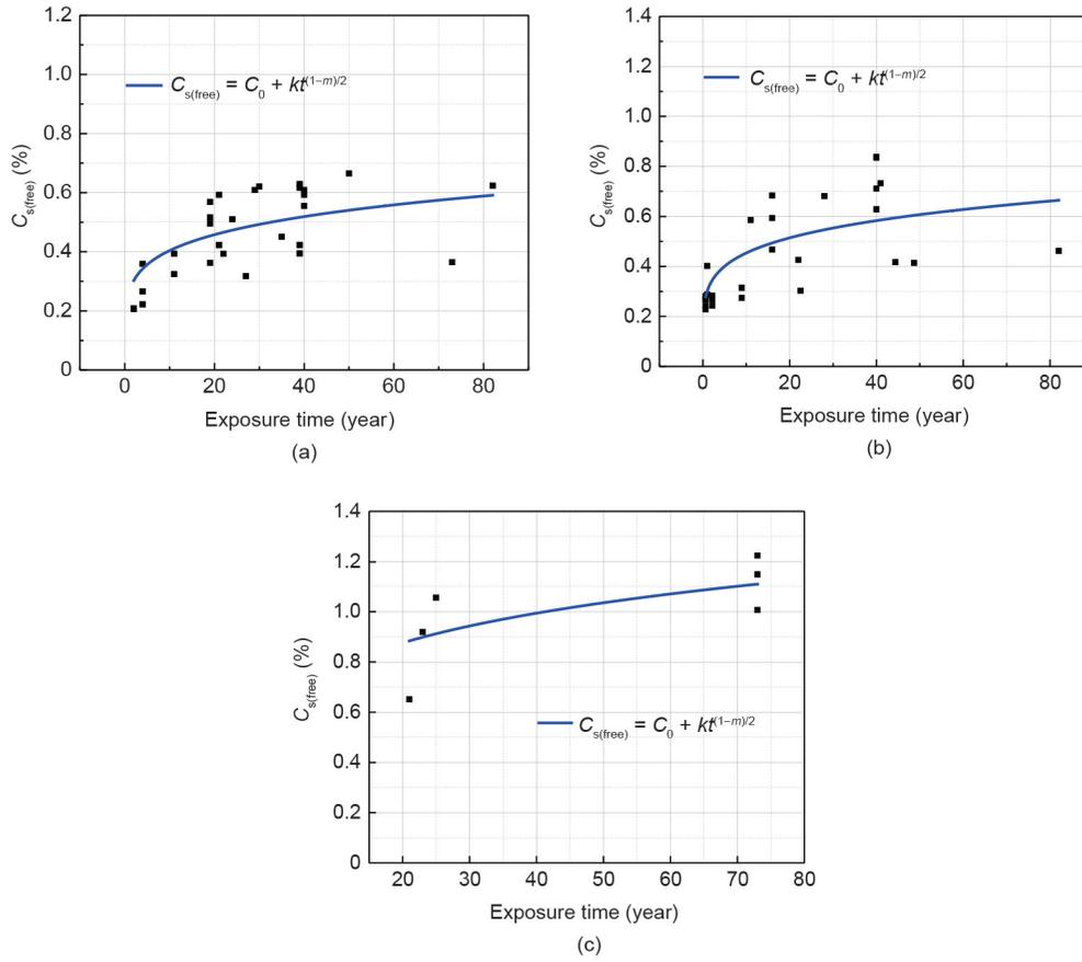
Fig. 9. Temporal variations in  $C_{s(free)}$  in different exposure zones. (a) Splash zone; (b) tidal zone; (c) underwater zone.
