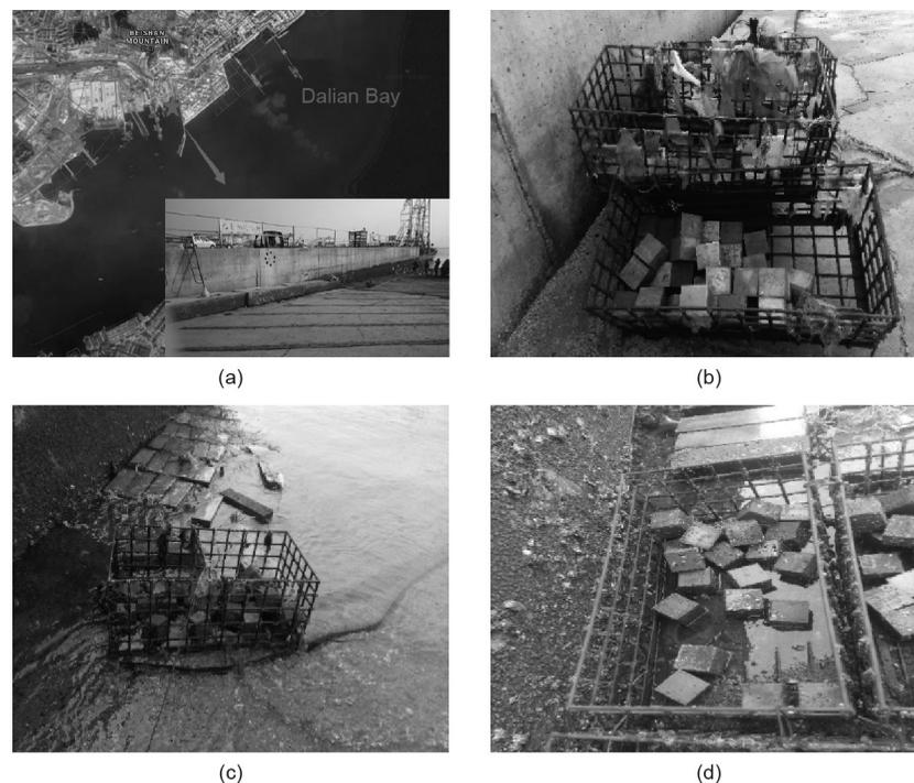
**Fig. 2.** Field exposure test. (a) Location of exposure station; (b) splash zone; (c) tidal zone; (d) underwater zone.
