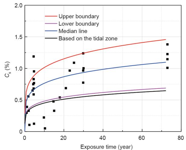
Fig. 17. Temporal variation in  $C_s$  in underwater zone in a global scale.
