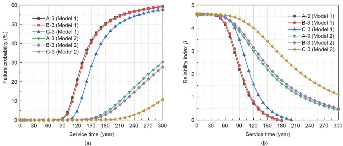
**Fig. 15.** Comparison of (a) corrosion probabilities and (b) reliability indices under two calculation conditions. Model 1:  $D_f$  decreases first and then remains stable, and  $C_s$  increases first and then remains stable; Model 2:  $C_s$  continuously increases and  $D_f$  continuously decreases.
