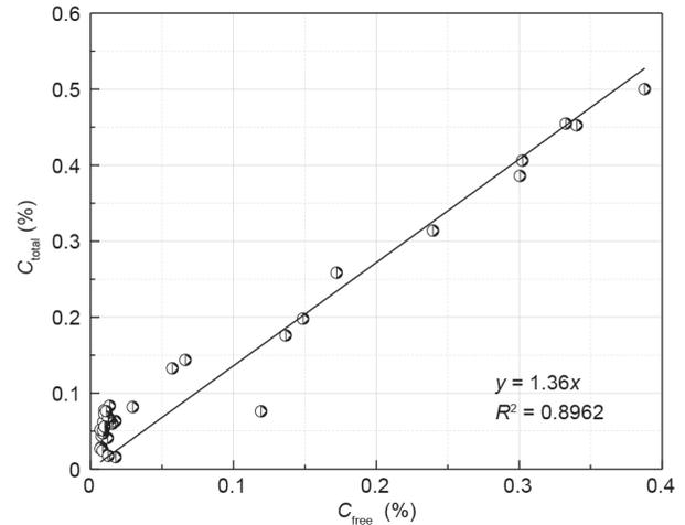
Fig. 6. Chloride binding capacity.
