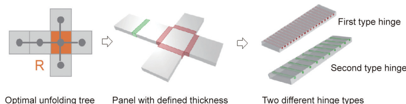
Fig. 7. Specific hinge design based on the optimal unfolding tree.
