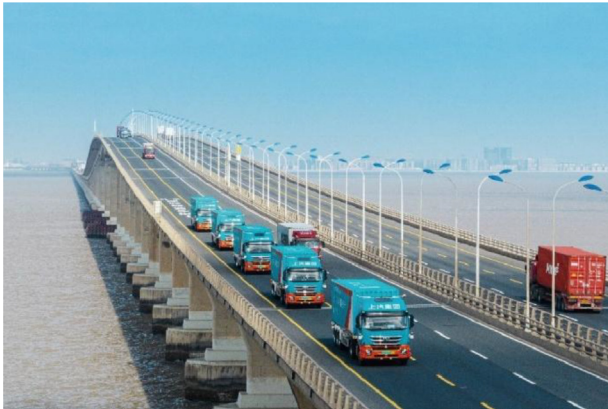
Fig. 1. Illustrative example of AVs (highlighted in blue) operating in a platoon amidst conventional traffic on China's Donghai Bridge.
