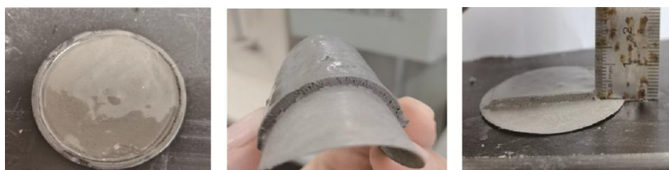
Fig. 12. The high-temperature and high-pressure filter cake (thin, dense, and tough, with a thickness of about 2 mm) of the superheat and salt resistant water-based drilling fluid system.
