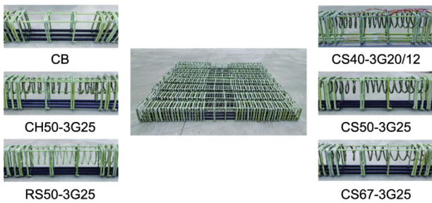
Fig. 2. FRP reinforcement cages of some of the test beams.
