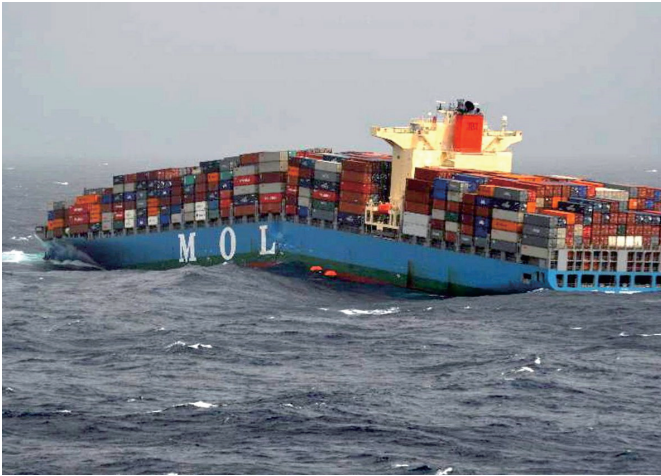
Figure 4. An example of a ship hull that was broken due to wave-induced stresses in the hull girder. ( http://www.rina.org.uk/mol_comfort_accident.html , 12 February 2015)
