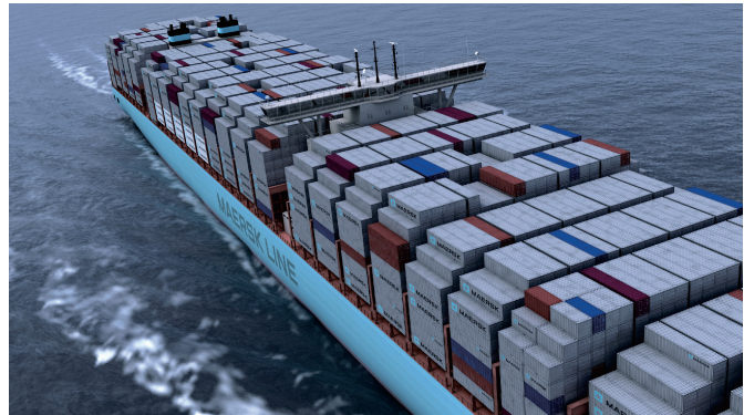
Figure 3. The Triple E. An example of the new generation of large container ships; it is 400 m long and 59 m wide, has a speed of 19 kn and carries 165 000 DWT. ( http://www.maersk.com/en/search?q=TripleE&t=images , 12 February 2015)
