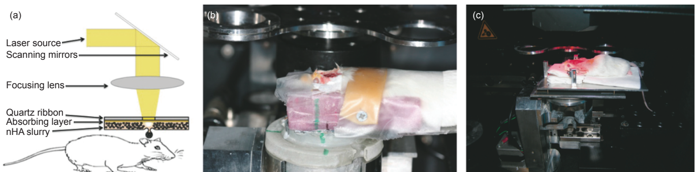
Figure 11. In vivo bioprinting using a BioLP system. (a) Illustration of operating setup; (b) mice placed in a specific holder; (c) the bioprinting process. (Adapted from Refs. [143, 144])
