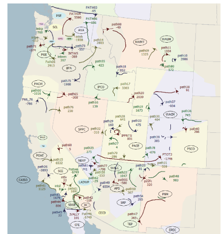
Figure 13. A WECC path flow visualization for a hypothetical operating condition.
