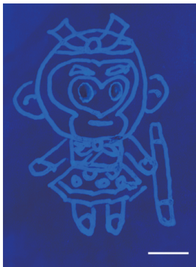
Fig. S5. Fluorescence photographs of FCD patterns after continuous irradiation under the UV lamp (365 nm) for 1 h; scale bar = 1 cm.
