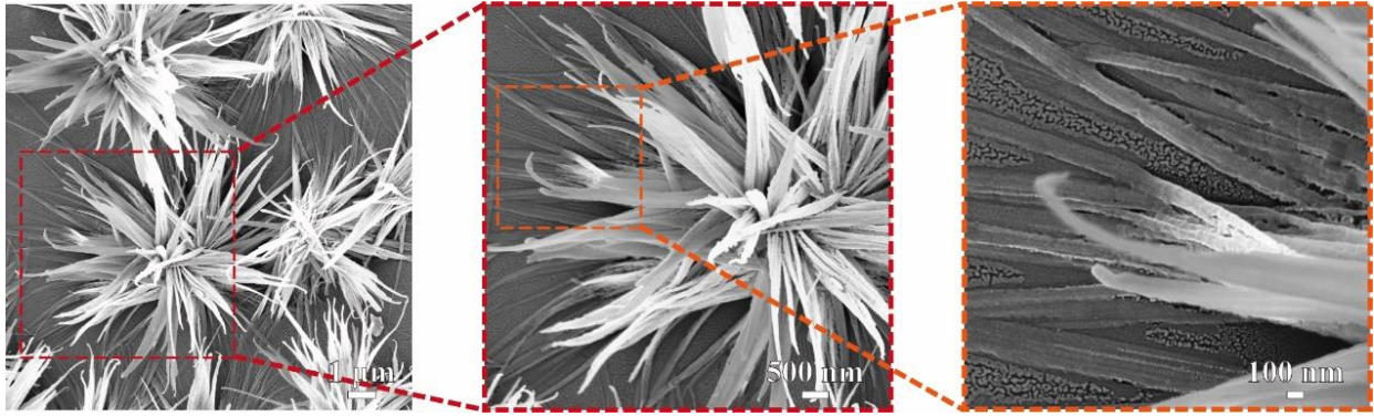
Fig. S3. SEM images of NPCs with typical morphology of “fibrous cluster-grooved skeleton” (taken from NPC3-600).
