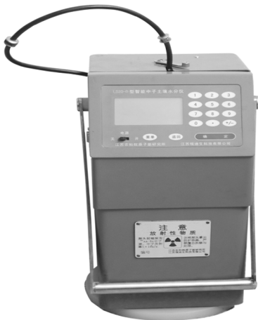
Fig. 4 In-hopper neutron moisture gauge of a type L250-D
