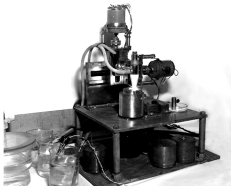
Fig. 3 Argon arc welding device
