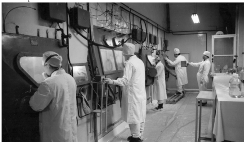
Fig. 2 Early work site of extracting 210 Po from irradiated Bi 2 O 3 targets
