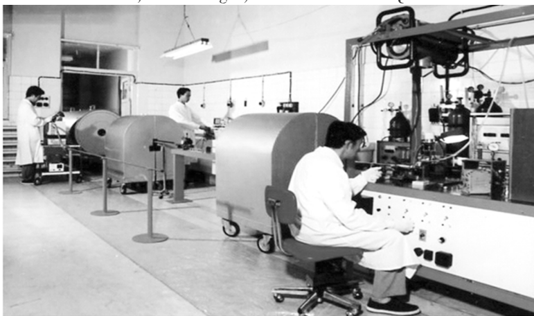
Fig. 16 Assembly line of neutron source rods
