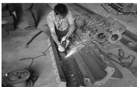
Fig. 4 Sandblasting inner surface of cable clip
