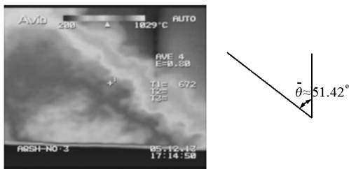
(c) The tilted plume for 0.7 m fire source
