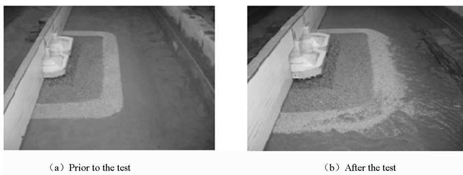
Fig. 3 Sketch of scour test of edge slope
