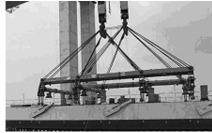
Fig. 5 Spreader structure with 8 lifting-points
