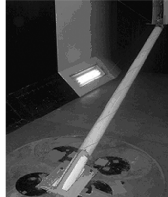
Fig. 8 1:1 model test for force measurement of Sutong Bridge
